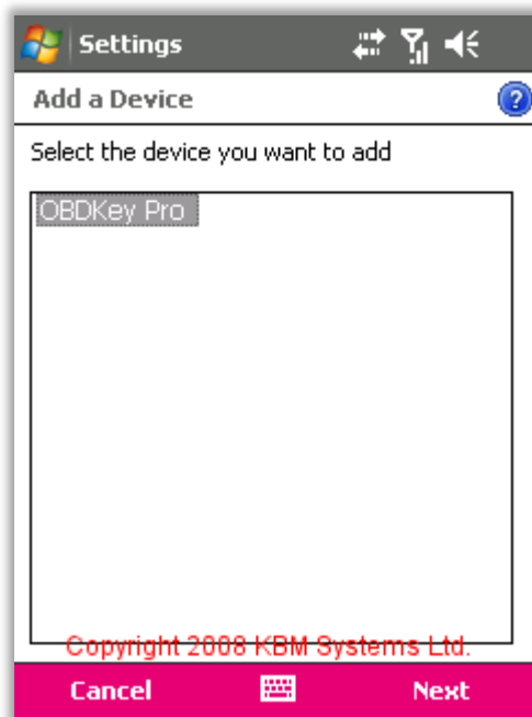
Figure 14 :: Bluetooth Settings –COM Ports – Add A Device - Tap “OBDKey Pro” then tap Next.
