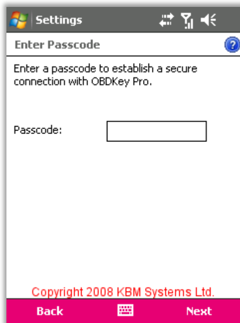
Figure 8 :: Bluetooth Settings –Enter Passcode for “OBDKey Pro” as 0000 (four zeroes)
