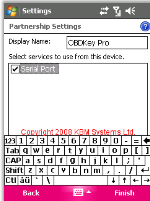
Figure 11 :: Bluetooth Settings –Ticked the Serial Port box. Tap Finish.
