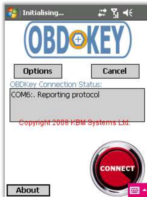
Figure 21 :: OBDGauge Connecting Status Screen. OBDKey will automatically detect which OBD protocol is used and best suited to you vehicle.
