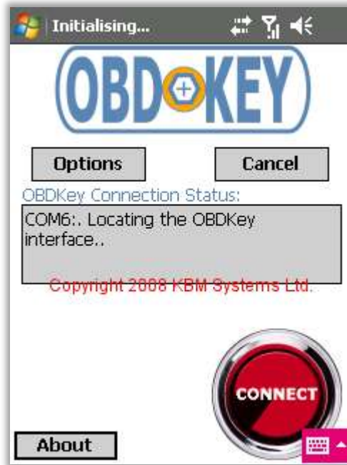
Figure 19 :: OBDGauge Connecting Status Screen. By default, OBDGauge uses COM6. If your outgoing serial port is not COM6, tap on the “Options” button.
