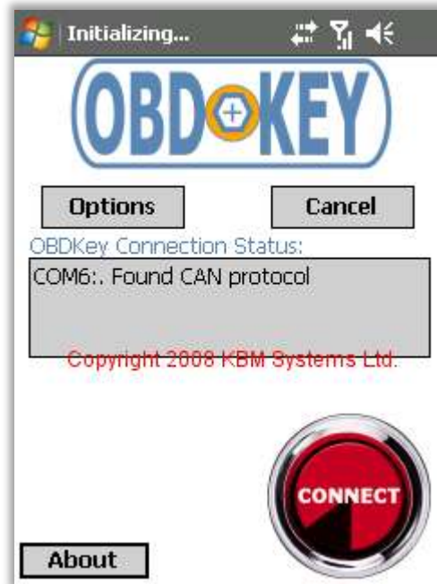
Figure 22 :: OBDGauge Connecting to OBD Key Status Screen. OBDKey will report which OBD protocol is to be used.
