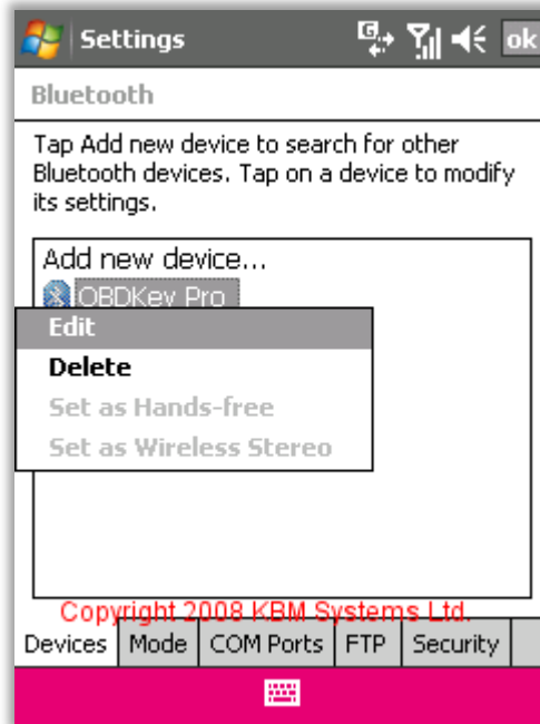
Figure 5a :: Bluetooth Settings – If your OBDKey is listed and you want to start the process again, tap and hold on the OBDKey listing item and tap the delete option when the menu appears.
